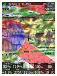
When **Show optimal track** is enabled, small blue arrow is drawn next to aircraft. This arrow indicates most optimal direction to fly.
