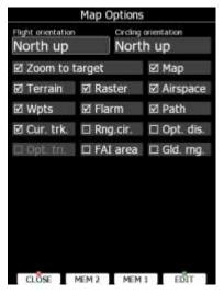
Map orientation is setup separately for straight flying or circling. If **Zoom to target** is checked the zoom will be automatically adjusted so that the target point is always visible. Maximum zoom is 200 km and minimum zoom is 1 km. The check boxes will turn on or off the following items:
