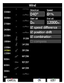
On rear seat device there is additional method called **front seat**. When **front seat** method is selected, device will use wind calculated by front seat only and all other methods will be disabled. This will ensure that both devices are using same wind for final glide calculations. The wind profile is shown on the left side of the dialogue. Yellow coloured altitude indicates our current MSL altitude. Using the ZOOM selector knob you can scroll up and down through the wind layers.
