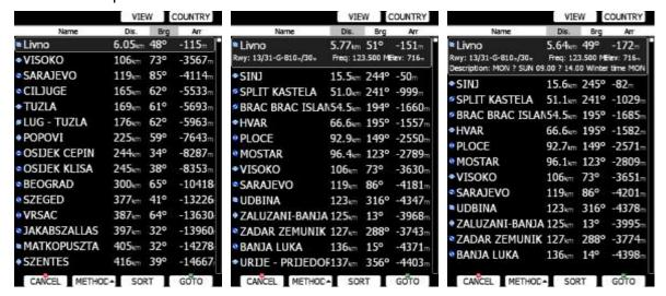
Press the **VIEW** button to change details of selected airport. Press the **SORT** button to change the sort order of the airports. Select an airport using the PAGE selector knob. Press **GOTO** and you will navigate to it. Press **COUNTRY** button and a dialogue window with a list of all available countries will pop up.
