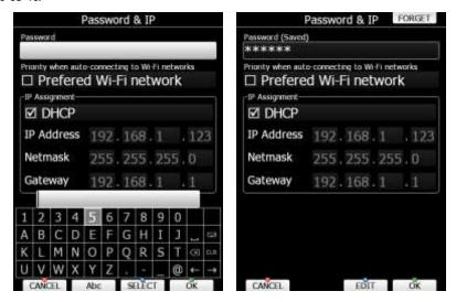
Use preferred Wi-Fi network option, if you would like to connect to this network only. Press **CONNECT** to connect to this network and press **FORGET** to forget this network.
