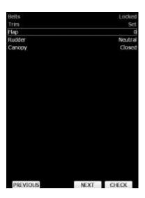
Checklists can be found at the last page of APT/WPT and TSK page. Once the action of the checklist is performed press the **CHECK** button. To move through the actions on the checklist use the **NEXT** or **PREVIOUS** buttons.
