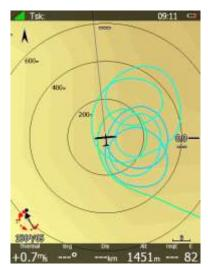
Previous navigational page will be restored when your aircraft will stop circling. You can also manually exit thermal mode by rotating PAGE or ZOOM knobs.
