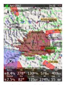
Use **Show glider range area** to display reachable area from current altitude with current wind and MacCready settings. Use **area colour** and **area border** to define its properties. Area can be filled outside or inside. **Glide ratio** defines the past flown average efficiency which will be used for average efficiency calculation for glider range area. Press the **DEFAULT** button to reset these settings back to default.
