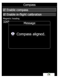
Press **CALIB** button to start calibration of compass on the ground. Calibration process I very straightforward. Make sure glider fuselage is levelled (use tail dolly), wings are levelled and canopy is closed with pilot inside. Switch on all the avionics, which is normally switched on while flying. Confirm calibration of compass to start calibration process. Assistant on the wing should slowly rotate glider with wings levelled.
