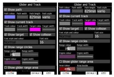
Check the **Show path** item if you want to see the flown path. **Path length** defines how much of the flown path will be shown. The path can be coloured using:
