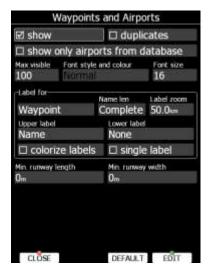
The **Max.visible** item defines how long waypoint labels and detailed symbols are shown. If the maximum number of waypoints on the current screen is more than the defined value only small blue dots will be shown for waypoints and no labels will be drawn.
