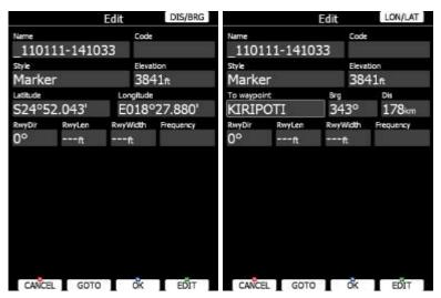
Waypoint data can be modified. Refer to Chapter 5.6.1 for more details. Press the **OK** button to save a marked waypoint or press **CANCEL** to exit without saving. Press **GOTO** button to navigate immediately to selected point.
