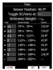
When all flap positions are set, a green dot will be displayed with current flap position. If flap labels are not set yet, press EDIT button to name flap label. Flap labels must me entered with increasing speed range. It is recommended that flaps labels are set together with speed range in Polar and Glider setup. See Chapter 0 for more details.
