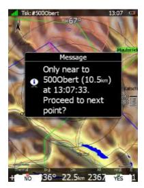
A message will appear. If you confirm this with **YES** the task will be advanced to the next turn point and it will recalculate the task taking the optimal fix as the task point.
