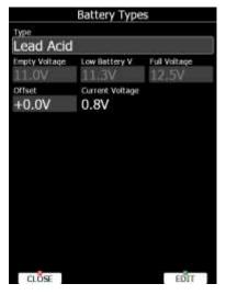
Use **Type** combo to select appropriate type of battery (Lead Acid, LiFe, LiPo, custom). You can see empty, low and full voltage for the selected type of battery. In case of voltage drop, because of cable lengths, you can set up voltage **offset** there to the **current voltage** measured.
