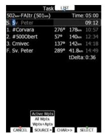
Pull down menu is used to select one of the options. Press button several times to select appropriate item of turn PAGE selector knob. Pull down menu will automatically close after few seconds.
