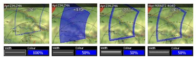
You can set separately airspace colour and border for side view and map view, if option **Copy styles to side view** is not checked. Press the **DEFAULT** button to reset these settings back to default.
