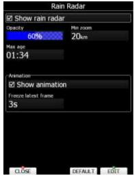
During flight, there is a possibility to get real time rain radar pictures, if Wi-fi module is connected to the 3g hotspot and if the hotspot has mobile signal.
