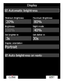
If the **Automatic brightness** checkbox is selected, the instrument will automatically adjust brightness according to current light conditions.
