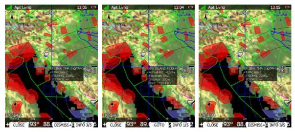
A blue cross will be plotted over the screen with info box for given cross position. Move cross up and down on map using PAGE selector knob. Move cross left and right using MODE selector knob. Turn ZOOM selector knob to zoom map.
