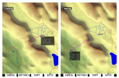
Details of selected airport will be drawn next to it. In upper-left corner of screen current sort method is shown. There are two possibilities, distance sort or bearing sort. Press **SORT** button to change it.
