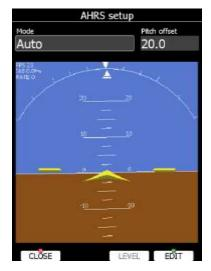
Place you glider in levelled position and press LEVEL button. You can also modify pitch offset, if you rotate PAGE selector knob. More detailed can be pitch set using pitch offset spin control.
