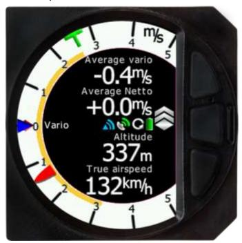
Indicator basic screen is split into two parts, white ring with needle and vario scale. Additionally to needle, blue MacCready triangle, green thermal average T and red diamond for 20 seconds average are shown. In the middle four user-customizable numbers are
