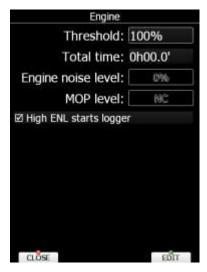
Set **Threshold** to define when engine is running. By default threshold is set to 100%, which means no engine run will be detected. Lower this value to approximately 80% to detect engine running. Engine total time will be accumulated and displayed in total time box. If necessary, total time can be adjusted, to match current engine total time. **High ENL starts logger** will start the flight recorder, if this option is enabled.
