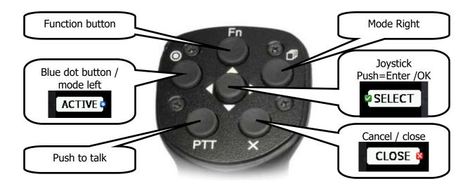
Remote stick has six push buttons and on multi-directional button in the middle. Move multi-directional button left and right to zoom in and out. Move it in up and down direction to select different page of to move on menu. Press it to select and item or to invoke a menu in navigational mode.
