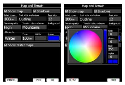
Rotating the zoom selector changes colour transparency. Transparency is very important for fill colours which are used for airspace zones, observation zones and FAI area. If a fill colour is not transparent (0%), all other map items will not be seen through it. If a fill colour is 100% only the solid border will be drawn.
