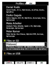
A profile can also be locked. This option is very useful for club operation where one does not want a global club profile to be changed. When a profile is locked all settings will be read-only. Press **LOCK** button to lock/unlock profile. When a profile is locked am message (locked) will be written below the profile name. Press **ACTIVE** to make selected profile as active one.
