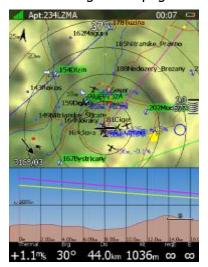
Side view is showing lateral view from glider towards selected goal. Terrain below glider is displayed including glider projected track based on glide ratio in grey colour. Yellow and magenta lines are showing requested glide ratio to goal based on zero MacCready setting and current MacCready setting.
