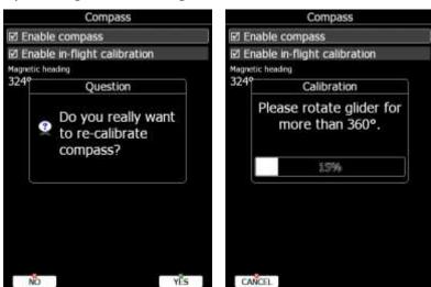
Keep rotating glider until progress reaches 100%. Calibration will automatically exit and compass calibration is finished. Check compass directions afterwards, they should be within +/-2 degrees. Press PTT on radio to see if there is any deviation in magnetic heading. If more error is observed, install compass in different place and repeat calibration procedure.
