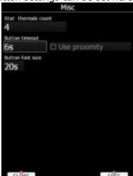
Screen button appearance can be set by **button timeout** time. For newest instruments proximity buttons can be used. Proximity will be detected after touch of a button if **Use proximity** is ticked. Also **button font size** can be set here.
