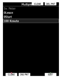
First start point will be grey out. This is point, which is defined in task. Add as many start points as required. Later it is possible to cycle through start points with CYCLE button.
