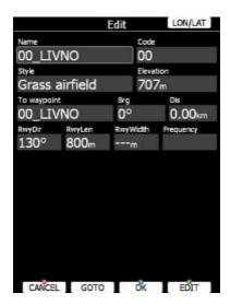
Press the **LON/LAT** button to toggle back to input of latitude and longitude. Modify other attributes at your discretion. When finished, press the **OK** button to confirm changes or press **CANCEL** to dismiss changes. The modified waypoint will be updated in the appropriate file automatically.
