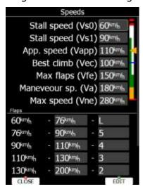
Once speed range is entered, the system will be able to display requested flap position based on current wing loading and g-factor.
