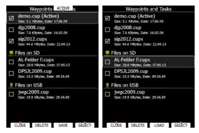
Multiple files can be selected. All checked files will be shown on the graphics page and used in the near mode calculation, if the waypoint is of the proper type (airport or outlanding place). However, only one file can be the active file. The active file is primary used for task creation. Task can be loaded only from the active file.
