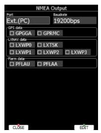
**Port** defines on which serial interface data will be transmitted. **Baud rate** defines transmission speed. Data is divided into three groups:
