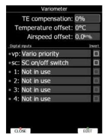
Total energy compensation, temperature offset, airspeed offset and digital inputs are setup in this menu.
