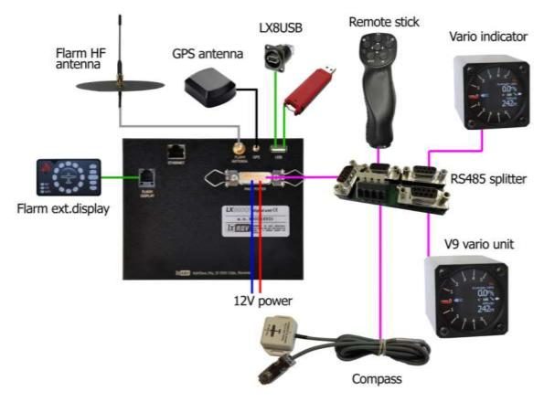
By using a RS485 bus system a wide range of optional interfaces can be easily connected to the basic configuration with minimal installation work. The LXNAV bus system can be extended easily by use of RS485 splitting units, which allow plug and play connection of optional devices.
