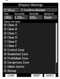
Airspace warnings are the most complex ones. An airspace warning is activated by two triggers; First warning (orange) will be given when a projected position of flight for period, which is defined in the **Time** item, is computed to cross an airspace zone.
