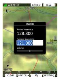
Press **SET FREQ** button to swap active and standby frequency. Press **SQ** to toggle volume control between **volume**, **squelch and vox**. Use upper left rotary knob to adjust it. In **HISTORY** pull down menu, a list of recently used frequencies is stored. Press **DUAL**, when available, to listen to active and standby frequency simultaneously. Press **8.33 KHz** to toggle between **25 KHz and 8.33 KHz** channel spacing.
