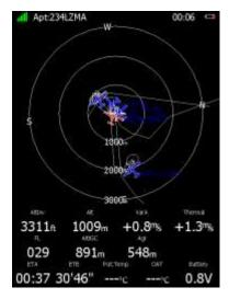
The internal pressure sensor altitude is shown as **AltIGC**. **AltInv** shows the altitude in opposite units to those defined in the **Units** setup. **OAT** is the outside temperature, **Pot.Temp** is the potential temperature and **Battery** displays the current voltage The estimated time of arrival and estimated time established are displayed at the bottom part of page.
