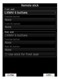
When a remote stick is connected to the system, it is possible to define type of remote stick via this menu. In case LXNAV remote stick with six buttons is connected, user can specify functionality of function button. There are several options available for function button:
