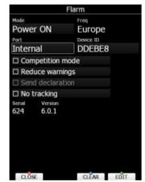
Press **CLEAR** button to delete all data on Flarm module. This will remove also obstacle database.
