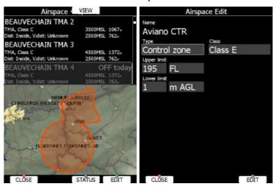
The **VIEW** button toggles the list views. When the **STATUS** button is pressed the status of the selected airspace zone will toggle between **OFF always**, **OFF today**, **OFF hh:mm** and enabled.
