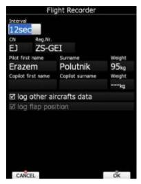
Select the recording interval and enter the pilot name. **Pilot weight is important if ballast is specified in kilograms of water** (see Chapter 5.1.9.5). If the system is used in two-seat aircraft the name of the co-pilot may also be entered.
