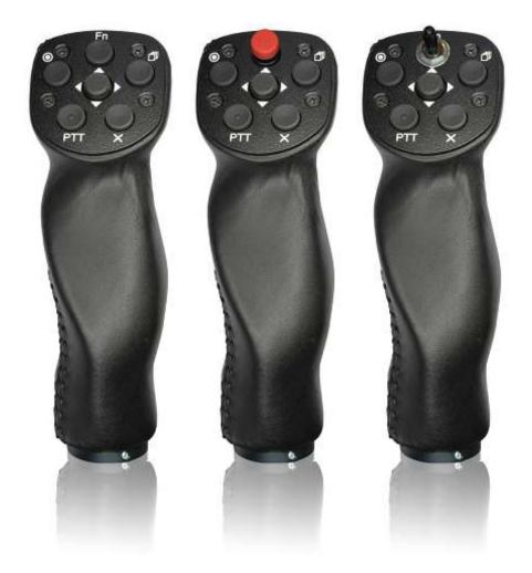
The stick is available also in various diameters: 18 mm, 19.3 mm, 20.3 mm, 24.4 mm and 25.4 mm. All necessary electronics is built into the top of the stick. The four coloured wires from the bottom must be connected to RS485 splitter. Additionally two shielded cables are used for speed to fly command and push to talk button.
