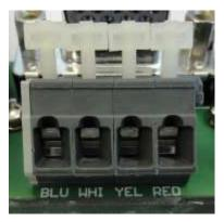
PTT wires are connected to radio push to talk input and SC wire is connected to Speed to fly input of vario unit.
