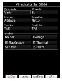
I8/I80 are not changing screen when toggling between cruise and climb mode. In setup you can define value for each line separately.
