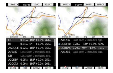
The list is sorted by distance. Device ID, distance, bearing, vario and altimeter parameters are displayed in the list. Lost target is still seen in the list showing when it was lost. Move through Flarm targets using PAGE selector button. Press **SELECT** button to mark selected target as favourite target. A yellow star will be drawn next to it. You can select as many favourites as you want.
