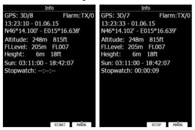
Press **START** button to start running stopwatch. Press **STOP** button to stop running stopwatch. If you press the **MARK** button a new waypoint will be created with the current latitude, longitude and elevation based on the terrain database. The waypoint name is generated from the current date and time separated by the minus character and preceded by an underscore.
