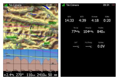
The first page is identical to first pages of the airport and waypoint modes. It shows navigational data to the current turn point. However the final glide indicator always shows the required altitude to complete the task.
