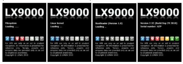
The boot procedure normally takes up to 20 seconds but in the case of a firmware update or system check it can take more time. The final boot screen displays information about the LX90xx system firmware and the IGC serial number. When the boot procedure is completed the profile selection dialogue is shown. Please refer to Chapter 7.1 for more details about starting up the system.
