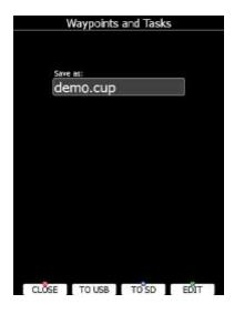
Change the filename if required. Press **TO USB** for saving to the USB stick or press **TO SD** for saving to the SD card.
