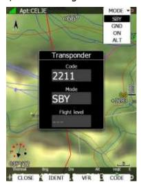
Use **MODE** to select mode of operation of connected transponder (**STBY, GND, ON, ALT**). Press **CODE** to enter squawk code. Press **VFR** to automatically set squawk code to 7000. Press **IDENT** to identify.
