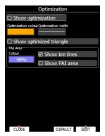
Check the **Show optimization** item to enable display of the optimised track. **Optimization colour** and **width** defines the colour and width for these lines.
