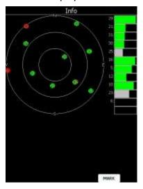
Green satellites are satellites currently being used for position determination. Three concentric circles represent satellite elevation (0, 30, 60 degrees above horizon). If a satellite is in the centre of the circles it is directly overhead.
