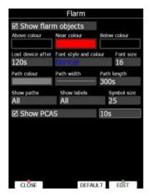
Checking **Show Flarm object** will enable display of aircraft detected by FLARM.
