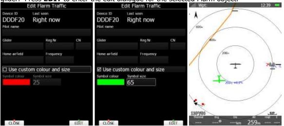
Enter data about the Flarm glider and pilot. The colour and size of each target can be adjusted by ticking the custom box.
