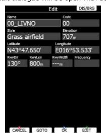
There are two possibilities to enter a position. You can modify latitude and longitude to define a position of the point or press the **DIS/BRG** button to enter the position as distance and bearing to a selectable point.
