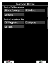
Data is divided into two groups; flight parameters and navigational data. If a specific value is checked this value will be automatically be received from the other device.
