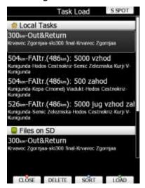
Total task distance, task description and task points are shown for each task stored. Select the desired task by rotating the PAGE selector knob and press **LOAD**. The task will be loaded into the active task and the task edit dialogue will be opened.
