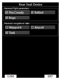
Data are divided into two groups; flight parameters and navigational data. If a specific value is checked this value will be automatically received from the other device.
