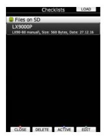
• Checklist is automatically added to the last page of the ATP/WPT and TSK screen.
