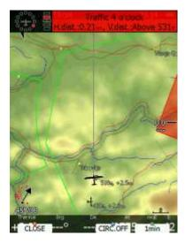
Picture above shows typical Flarm warning with graphical presentation and relative bearing of object. Press CLOSE to dismiss warning, CIRC.OFF to dismiss for time of circling and 1min to dismiss all Flarm warnings for one minute.
