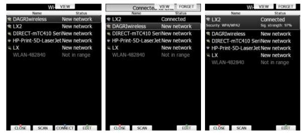
Press **SCAN** to scan for new networks. Use **EDIT** to enter password for selected network and to connect to it.
