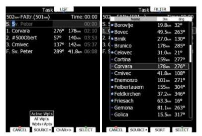
Sometimes, it is easier to see list of all waypoints. Press **LIST** button to change selection method to list mode. Press **FILTER** button to go back to this mode. In list selection mode, it is possible to **SORT** waypoints on name, distance or bearing. Distance and bearing are calculated to previous point in task. This is very useful, when you do not know exactly waypoint name, but just direction and distance, where to go.
