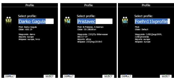
Turn the PAGE selector knob to select the desired profile if more than one profile is available. First profiles stored in internal storage are displayed, next profiles on SD card are shown and at last profiles on USB stick are shown. You will note profile resides on SD card/USB stick with small SD card/USB stick symbol in lower right part of pilot icon.
