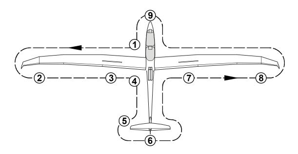
When walking around the Arcus T, check all surfaces for paint cracks, dents and unevenness. In case of doubt, ask an expert for advice.
