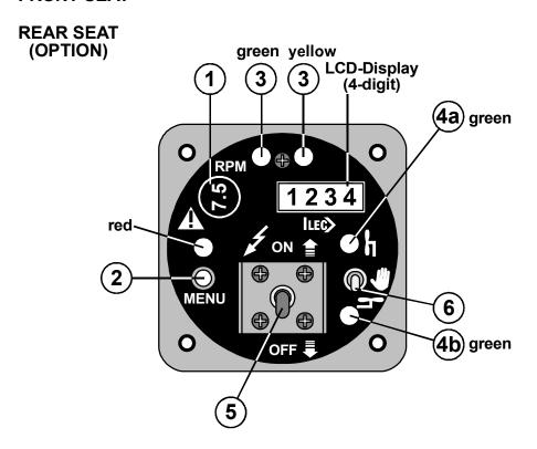
The engine control unit TB 06 is designed for a partially automatic extension and retraction procedure of the power plant for engine operation.
